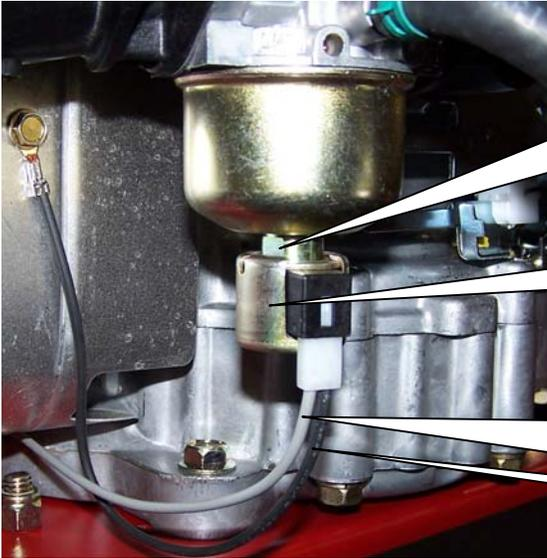
Very thin 1/2" wrench needed to remove this solenoid. **Do not** try to remove by using a pair of pliers on the coil section. Coil can be damaged very easily.
