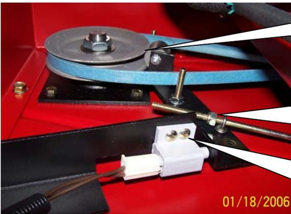
Belt can be tightened by turning the nuts clockwise on both sides or this angle bracket.
