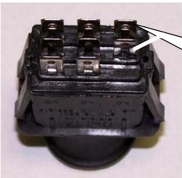
Some of our clutches have a different receptacle for the wiring harness, but the testing is the same. The white wire is always the negative terminal and the brown wire is the positive.
