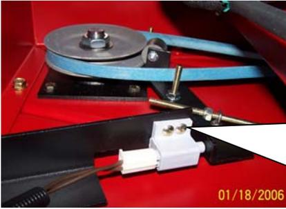
A neutral switch is located on the right side in the belt housing. The plunger button must be depressed at least 3/8 inch when the blades are disengaged. This can be adjusted by loosening the two mounting screws and sliding the switch to the side. Ohmmeter should go to zero when checking continuity across switch terminals with plunger depressed.
